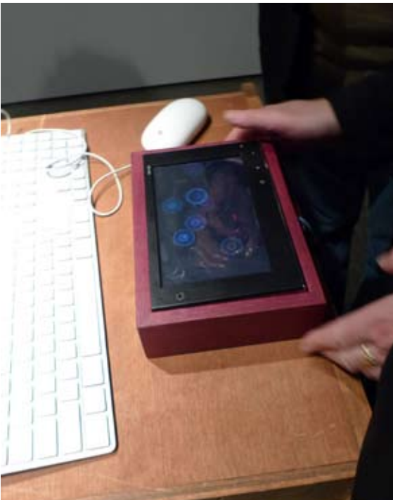
A tabletop version of shapeMix. The form factor of the small box allows a user to tip the box to move the shapes with an accelerometer.
